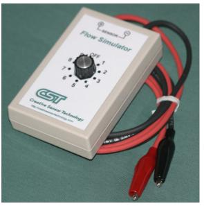
The CST Flow Simulator provides a practical way to simulate the output signal produced by CST and other two wire impeller type flow sensors.
